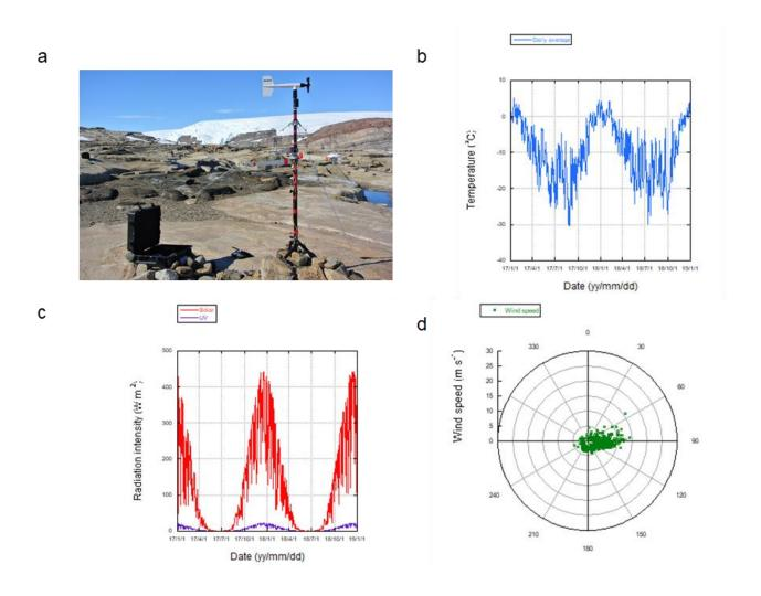
Figure 4. Skallen AWS (a) and examples of the graphical expression of daily averaged data of air temperature (b), solar and UV radiations (c), and wind conditions (d) recorded at Skallen from 1 January 2017 to 31 December 2018.
