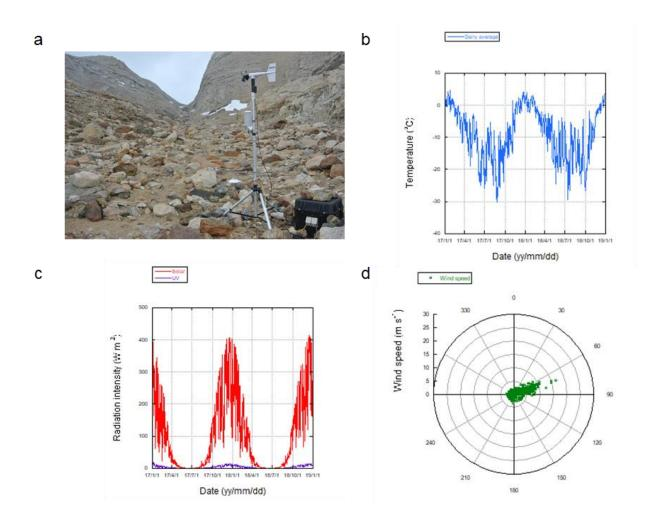
Figure 2. Yukidori Zawa AWS (a) and examples of graphical expressions of daily averaged data of air temperature (b), solar and UV radiations (c), and wind conditions (d) recorded at Yukidori Zawa from 1 January 2017 to 28 December 2018.
