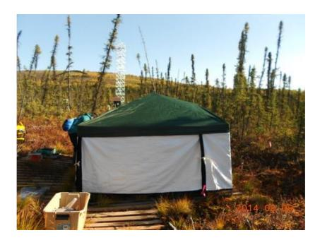
Fig. 4. The outdoor canopy with black curtains for the spectral reflectance measurements.
