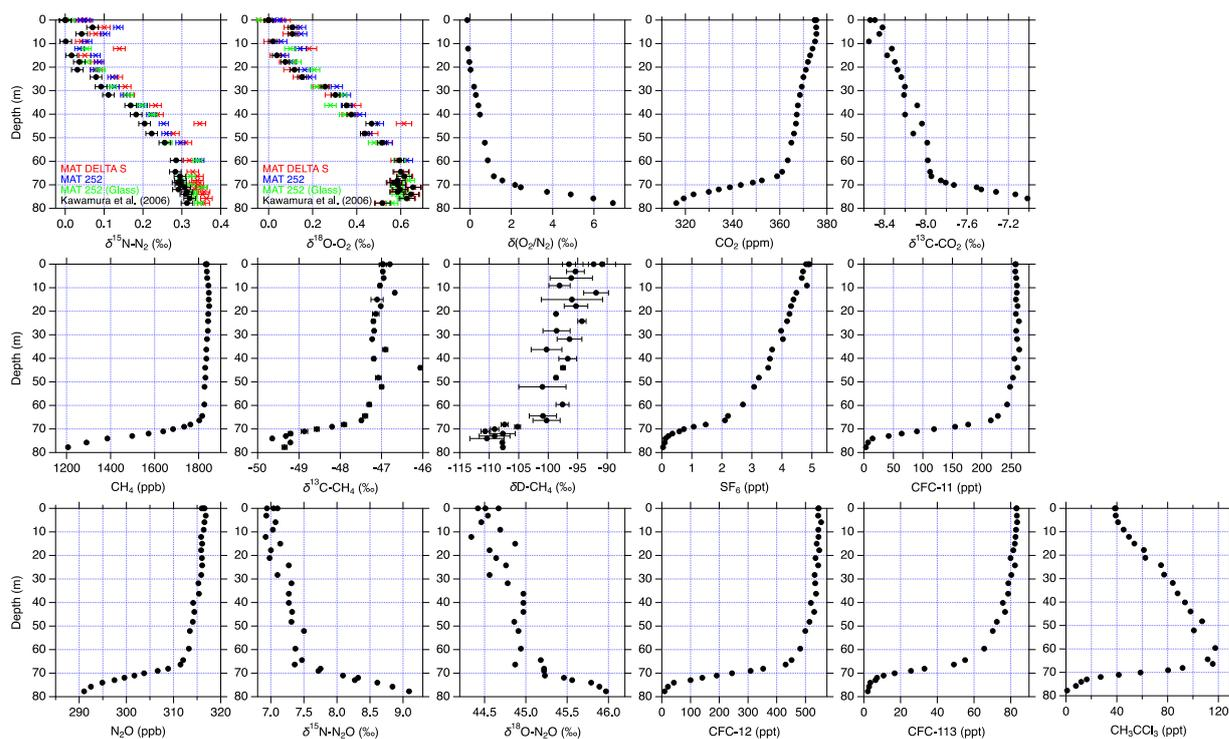
Fig. 2. Depth profiles of air composition and isotope ratios in the NGRIP firn.
