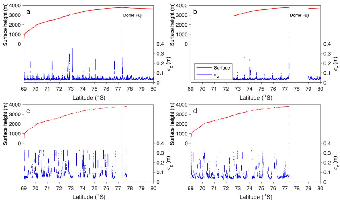
Figure 4. Surface height (red line) and the accuracy of GNSS measurements in the vertical direction ( $\sigma_z$ , blue line) along the surveyed route from (a) S16 to S80 during the 54th expedition, from (b) S80 to S16 during the 54th expedition, from (c) S16 to the BC during the 60th expedition, and from (d) the BC to S16 during the 60th expedition. Dashed lines indicate the location of Dome Fuji.
