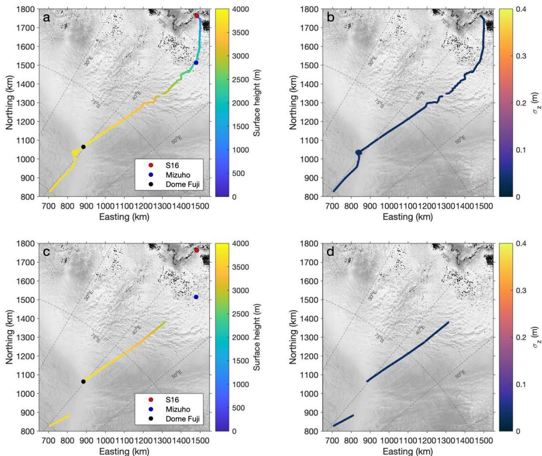
Figure 2. Surface height along the survey routes measured from (a) S16 to S80 and from (c) S80 to S16 during the 54th expedition. The accuracy of the kinematic GNSS measurements in the vertical direction ( $\sigma_z$ ) along the survey routes from (b) S16 to S80 and from (d) S80 to S16 during the 54th expedition. The background is a RADARSAT-1 image taken in 1997 (©CSA, 1997).
