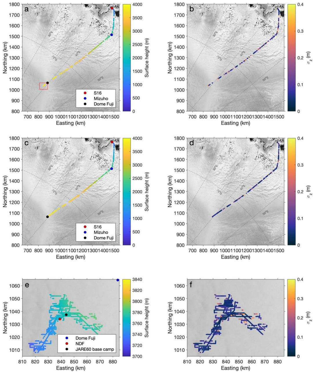
Figure 3. Surface height along the survey routes measured from (a) S16 to the basecamp (BC), (c) areas around the BC and NDF, and from (e) BC to S16 during the 60th expedition. The accuracy of the kinematic GNSS measurements in the vertical direction ( $\sigma_z$ ) along with the survey routes from (b) S16 to the BC, (d) areas around the BC and NDF, and from (f) the BC to S16 during the 60th expedition. The background is a RADARSAT-1 image taken in 1997 (©CSA, 1997).
