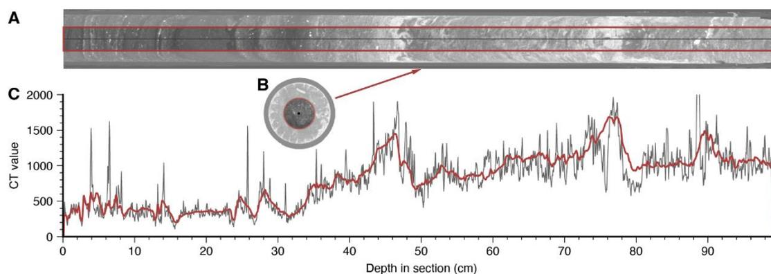
Figure 4. CT scanning image and CT values of NRM08 Section 2 using Pydicom. (A) and (B) CT image of NRM08 Section 2. The black line is the centerline of the CT values. The red shape is the area of average CT values. (C) The variation of CT values. The black line is the value of the centerline. The red line is the average CT value of the red shape in (A) and (B).
