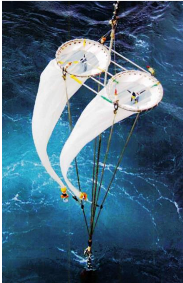
Fig. 3. The twin NORPAC standard net. Flow-meter is attached at each mouth ring of net.
