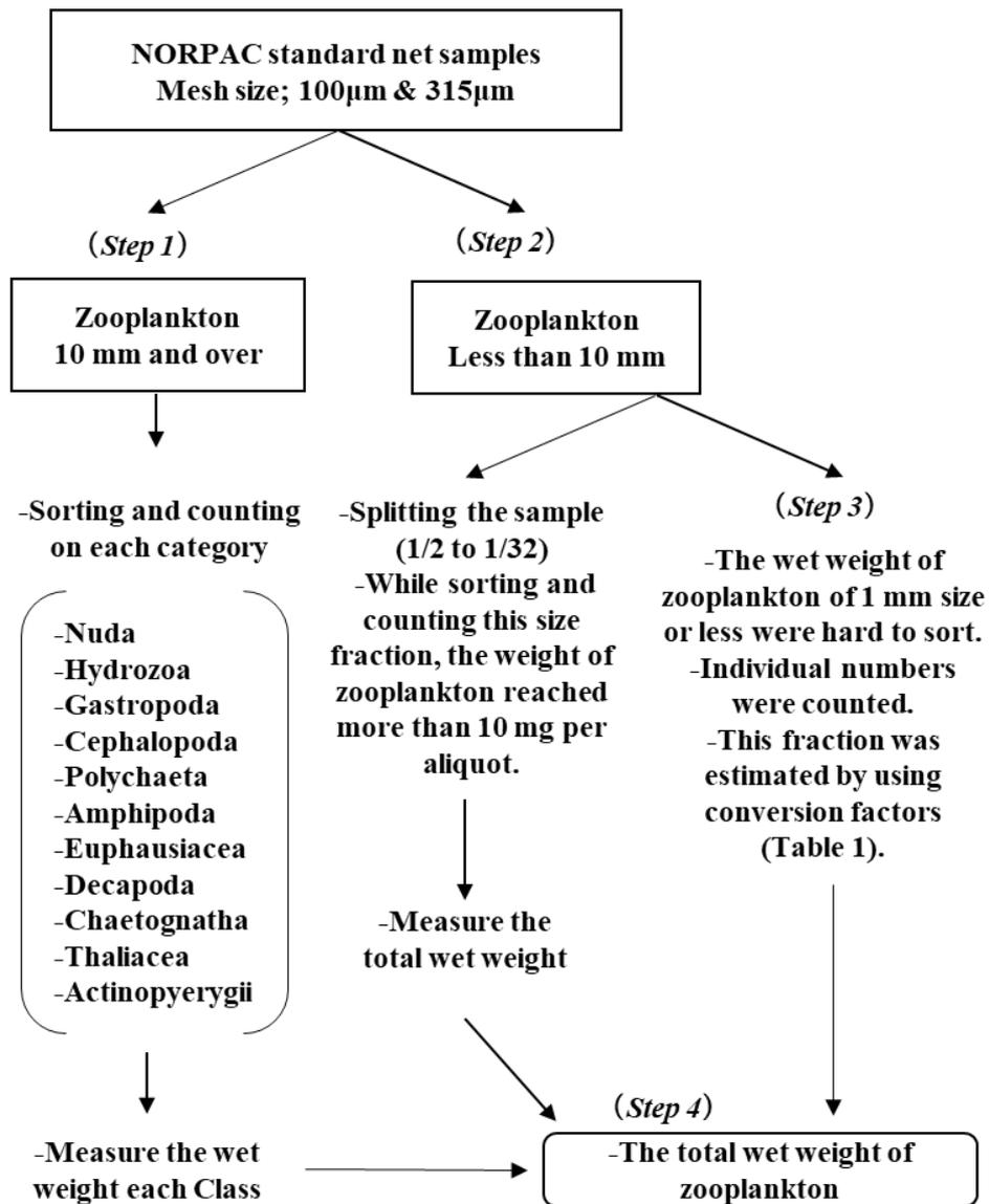
Fig. 4. Four-step procedure used to measure and to estimate the wet weight of NORPAC net samples.
