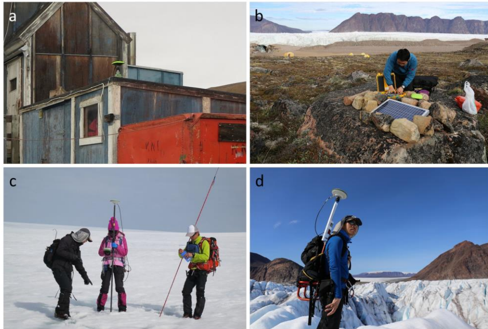
Figure 2. GPS reference stations in (a) Qaanaaq Village and (b) Bowdoin Glacier. Kinematic GPS measurements on (c) Qaanaaq Glacier in 2013, and (d) Bowdoin Glacier in 2015.
